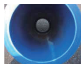
Inside of PE pipe used for nine years
