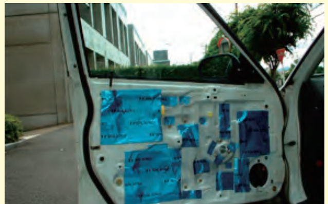
※Usage of REAL SCHILD: REAL SCHILD, the specialized vibration absorbing sheet for the improvement of sound quality of car audio systems, is a sister product of Calmmoon Sheet.
