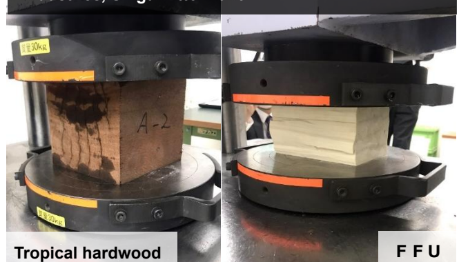
A compression test conducted at Sekisui Chemical Industries, Shiga Ritto Plant
